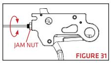
(FIGURE 31). Turning the screw clockwise will reduce the over travel and counterclockwise will increase the over travel.
