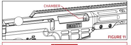
▲ WARNING DO NOT STORE OR TRANSPORT A LOADED RIFLE. ALWAYS REMOVE THE MAGAZINE AND CHECK THE CHAMBER TO ENSURE THE RIFLE IS UNLOADED.
