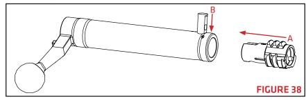
Insert the firing pin assembly into the bolt tube(FIGURE 39-A) and rotate clockwise to lock the firing pin assembly into the cocked position (FIGURE 39-B).
