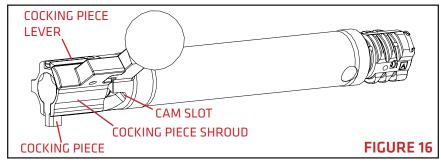
2. Rotate the cocking piece lever forward until it rests against the cocking piece shroud (FIGURE 17).
