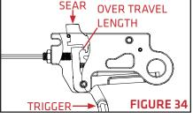
Turn the over travel screw clockwise until it locks up the trigger against the sear (FIGURE 35).
