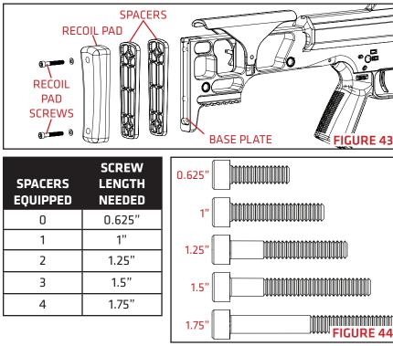
NOTE: USING THE WRONG LENGTH RECOIL PAD SCREWS WITH SPACERS COULD CAUSE INTERFERENCE WITH THE STOCK.
