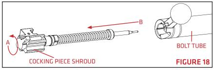
NOTE: IF THE COCKING PIECE LEVER BECOMES DECOCKED WHILE REMOVED FROM THE BOLT BODY, INSERT THE FIRING PIN ASSEMBLY BACK INTO THE BOLT TUBE (FIGURE 19-A). MANUALLY COMPRESS THE FIRING PIN SPRING AND ROTATE THE COCKING PIECE SHROUD BACK INTO THE ASSEMBLED/COCKED POSITION (FIGURE 19-B).
