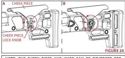
NOTE: THE CHEEK PIECE AND KNOB CAN BE REVERSED FOR LATERAL ADJUSTMENT.
